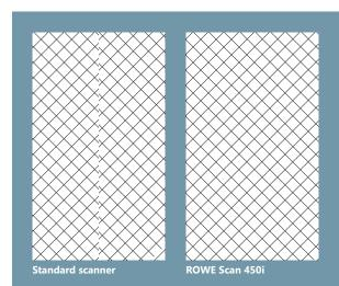
■ ROWE DYNAMIC STITCHING (RDS) (patent) ROWE engineers have achieved a groundbreaking innovation: excellent scans, even when the document is folded or thin. The patented ROWE DYNAMIC STITCHING continuously controls the scanned document data of each sensor and sets them together in real time. Any deviations that may occur are corrected automatically. Compare the difference!
